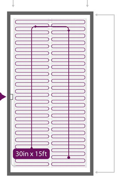
Cut the white mesh to shape the mats to fit any room. Any combination of mat sizes can be used up to 150 square feet per thermostat.
